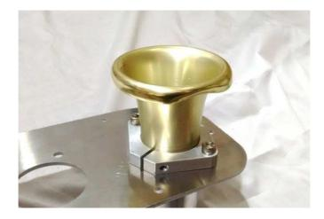
3) Assemble the two end trumpets and spaces to the backing plate with the clamping screws to the inside and the folded lip to the bottom of the last cylinder. Leave the bolts finger tight
