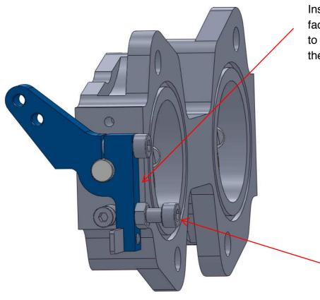
Install master lever with back face perfectly vertical or parallel to the back face of the ITB when the throttle plates are fully closed
